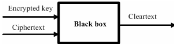
Fig. 1. Black-box model with inputs of encrypted key and ciphertext and it outputs cleartext
